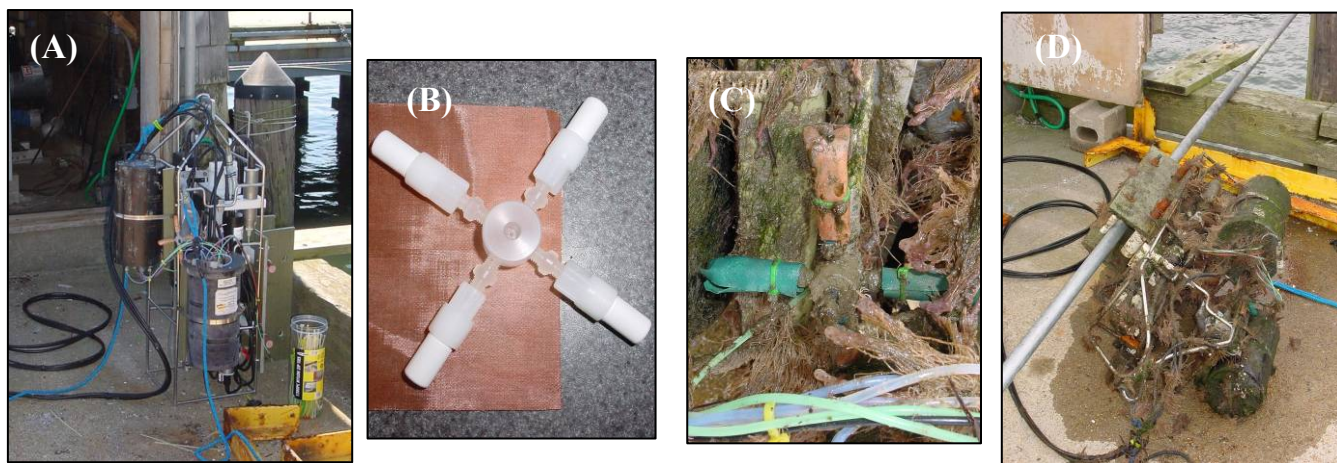
Fig. 3 (A) URI-GSO Pier Sampling Package during 9/9/2008 pre-deployment. Package includes the APNA with reagent reservoir, Sea-Bird SBE 911 CTD with DO and pH probe, and WET Labs’ WetStar [Chl a] Fluorometer and AStar Transmissometer. (B) 4-Filter (10µm) Sampling Head and copper mesh during 9/9/2008 pre-deployment. (C) 4-Filter Sampling Head upon 9/30/2008 retrieval. (D) GSO Pier Sampling Package upon 9/30/2008 retrieval.
